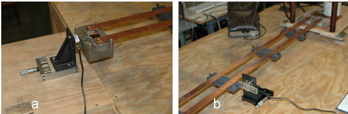
Figure 16. Lorentz force armature load cell (a), recoil force load cell (b)
